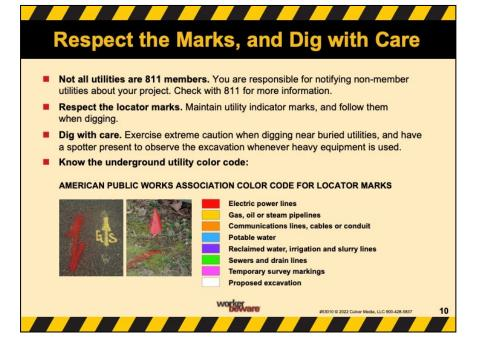
After you contact 811, the underground utility locator service will arrange for each member utility to send someone out to your dig site to mark the underground lines.
